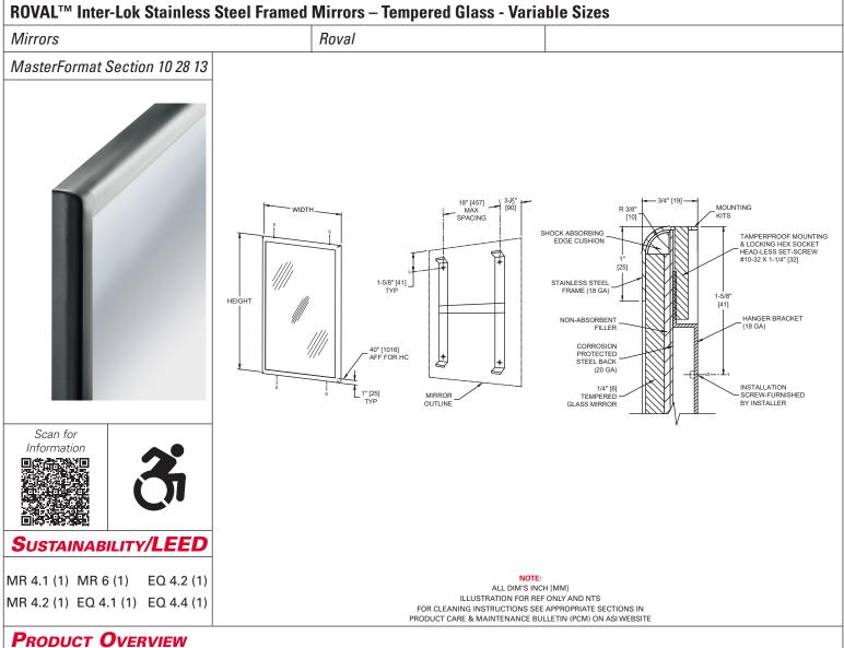
Gently radiused edges match the ASI Roval<sup>™</sup> design. Frame fabricated of 18 gauge type 304, alloy 18-8 stainless steel with satin finish and polished seamless mitered corners. 0.25" [6.4] thick tempered glass mirror. See Price List for all sizes available. Variable sizes available.
